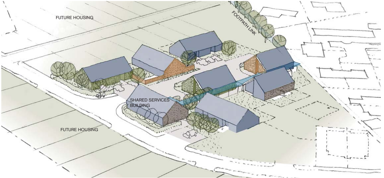
Above Site perspective This image Each building has two larch elevations, and two where the slate roof runs down to the ground Right The houses are connected through footpath links
